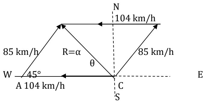
$$\begin{aligned} a &= \sqrt{b^2 + c^2 - 2 \times b \times c \cos A} \\ &= 85^2 + 104^2 - 2 \times 85 \times 104 \cos 45^\circ \checkmark \\ &= 74,427 \text{ km/h} \checkmark \end{aligned}$$
