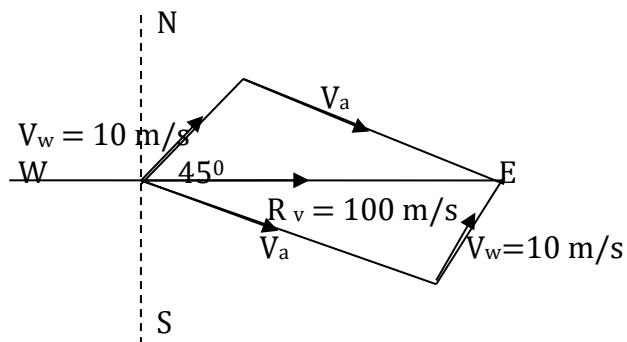
$$V_a = \sqrt{V^2 + R^2 - 2 \times V_w \times R_v \cos A} \checkmark$$
