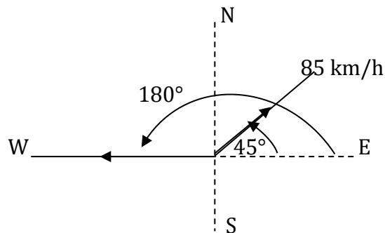
$$\begin{aligned}\sum V &= 85\sin 45^\circ + 104\sin 180^\circ \\ &= 60,104 \text{ km/h} \checkmark\end{aligned}$$
