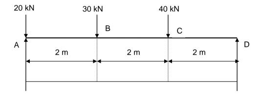
4.2.1 Calculate the reaction forces at the support A and D, and test the answer. (4)
